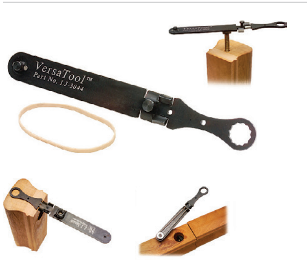
3044 Versa Tool Our VersaTool locates holes as well as starts and tightens hex nuts onto rail bolts. Drives 5/16" rail bolts and tightens 1/2" hex nuts. Also used to locate 1/4" pilot hole on handrails & rail drops for attaching to Conect-A-Kit® handrail fittings
